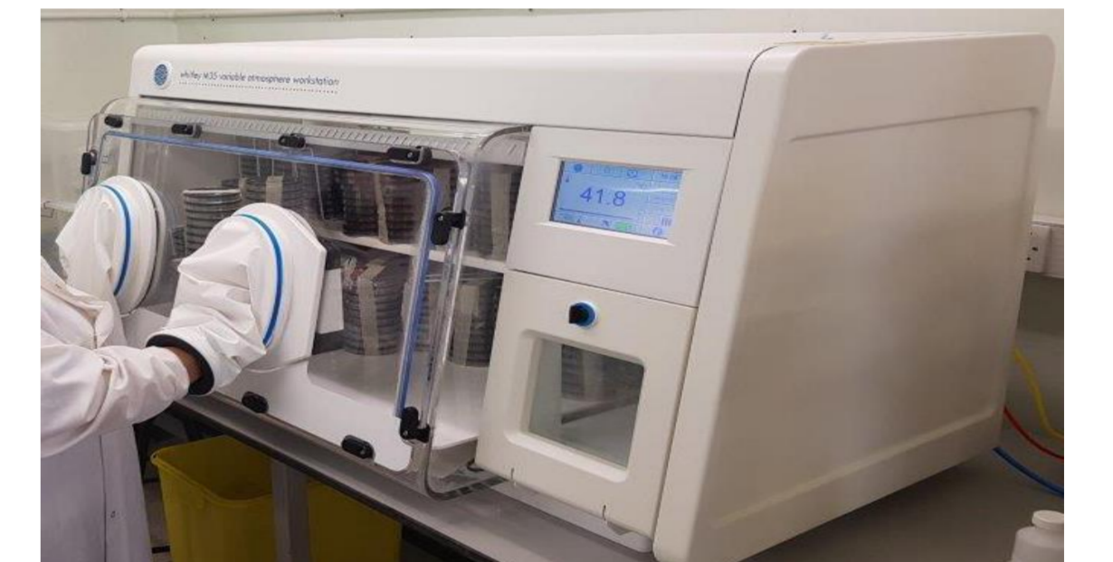
Figure 4: Don Whitley DWS M35 cabinet. Viable count of recovered colonies in a Don Whitley M35 cabinet, at 42°C for 48h, in a microaerophilic atmosphere of 5% O 2 , 5% CO 2 , 2% H 2 and 88% N 2
